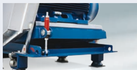
Easy to use: multifunctional hinged motor mount lifting jack from AERZEN
