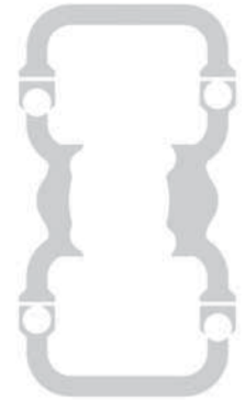
FIGURE 3 At completion of the stroke, the air valve again redirects air to the back side of diaphragm A, which starts diaphragm B on its exhaust stroke. As the pump reaches its original starting point, each diaphragm has gone through one exhaust and one discharge stroke. This constitutes one complete pumping cycle. The pump may take several cycles to completely prime depending on the conditions of the application.
