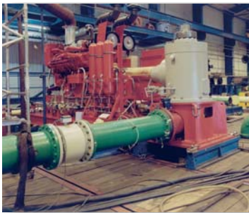
SPP Vertical Turbine pump on test at the Coleford manufacturing facility
