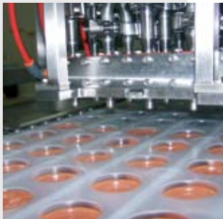
PCM dosing accuracy is +/- 0.5%
