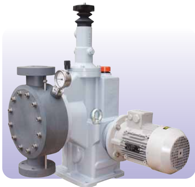
< XLC PVC basic version with: double diaphragm with local visual rupture detector and flanged con- nections.
