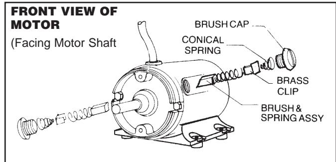
Replacement brush kit includes 2 each brush and spring assemblies, brass clips, conical springs, and caps.
